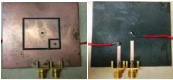
Fig. 2 Fabricated antenna. Top view (ground plane side) on the left and Bottom view (feed line and bias side) on the right.
